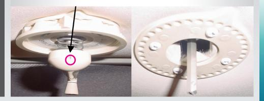
Remove sealant & screws from base, remove antenna and clean surface
